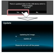
**Caution:** The screen may go blank for a few seconds. Do not unplug the USB memory or Power Off the unit during the Update Procedure.
