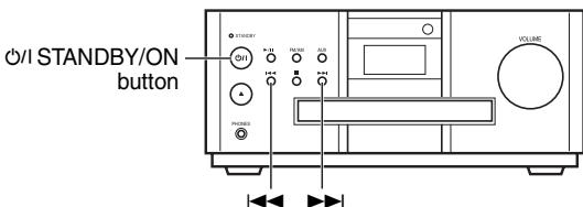
To select 10 kHz intervals, while holding down ►► on the main unit in Standby mode, press O/I STANDBY/ON on the main unit to turn on the power. "10 kHz" appears on the display window.
