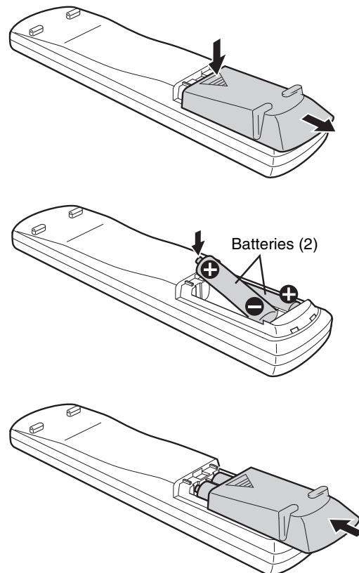
If the range or effectiveness of the remote control decreases, replace the batteries. Use two R6P (SUM-3)/AA(15F) type dry-cell batteries.
