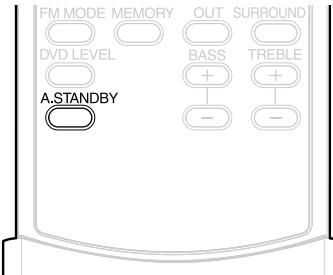
If there is no operation for 3 minutes while the disc is stopped, the power will be automatically turned off.
