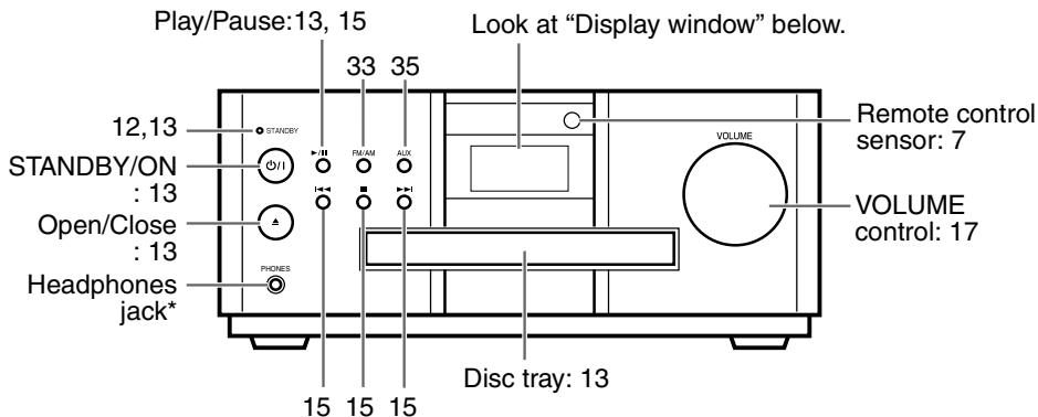
\* Connect a pair of headphones (commercially available) with a stereo mini plug. If the headphones are connected, the speakers and subwoofer will not produce any sound.
