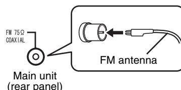
Put the antenna up straight in the direction where the best radio reception can be obtained, and fix by using tape.
